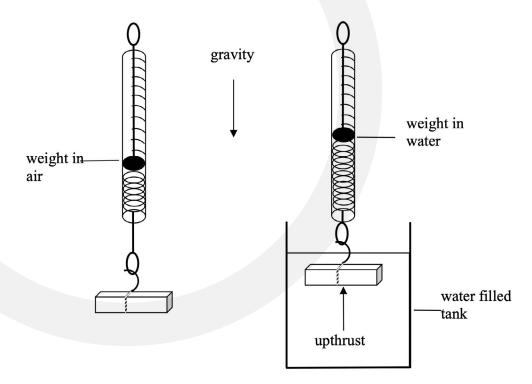
Weighing an object to find the effect of up thrust in water.
